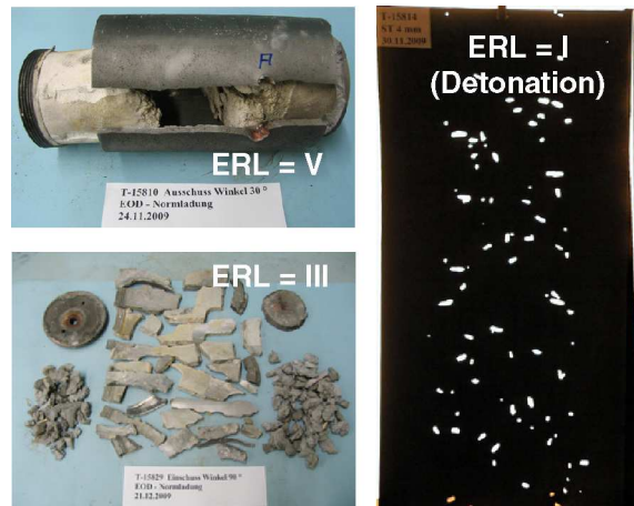
Fig. 4: Typical explosive reaction levels (ERL) achieved during the SCJ initiation tests.
